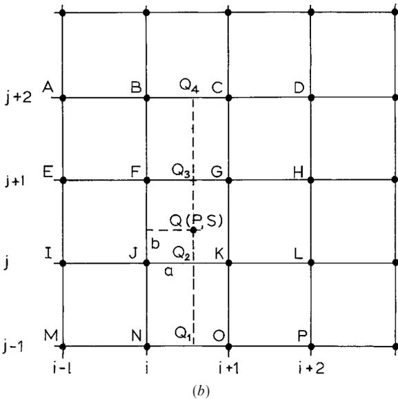
Figure 10. Grid for the definition of a resampling formula (a) for bilinear interpolation, and (b) for bicubic interpolation.
