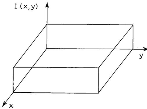
Figure 4. Idealised response function (point spread function).
