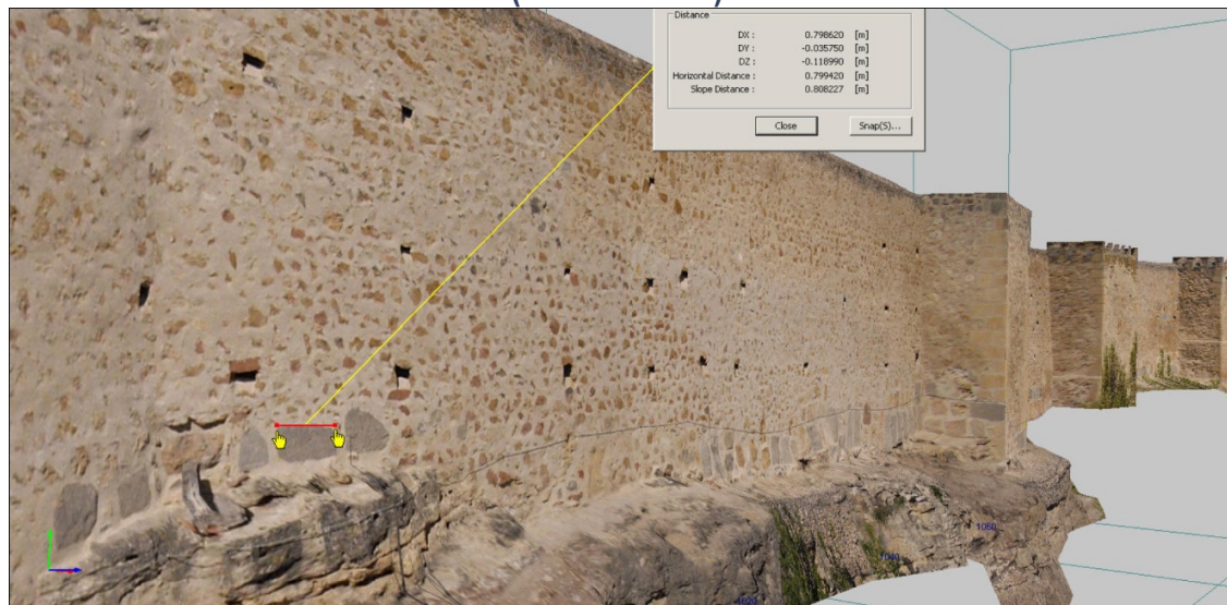
I.e. – Measurement of dimensions in masonry elements, over the 3D model
